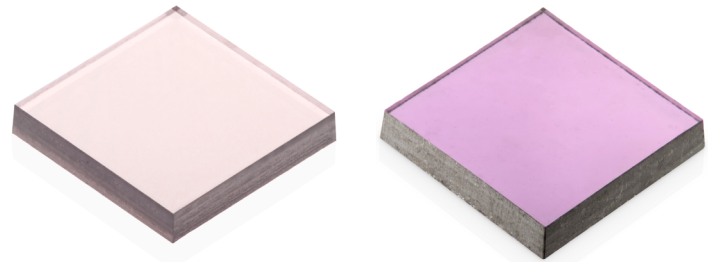
Figure 2: DNV B1 (left) and DNV B14 (right) CVD diamond samples
